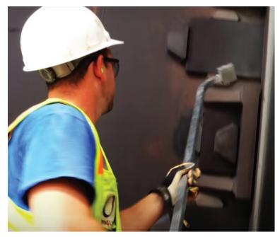
Our lightweight, 5-feet-long Easy Bar® Lubricator insertion tool has a flexible neck that can be easily angled for swift application. The tool is specially designed to firmly hold any Easy Bar without interfering with the release of the bar.
